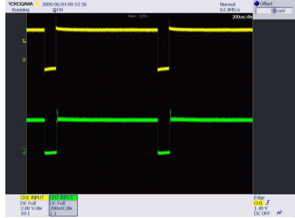
V_{IN} = 4.2\text{ V} , Ch1 – PWM, Ch2 – LED current (400 mA/div)
