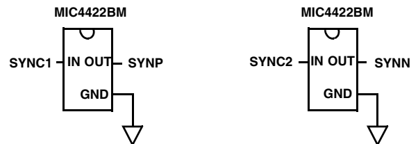
FIGURE 22B. NON-INVERTING DRIVERS
