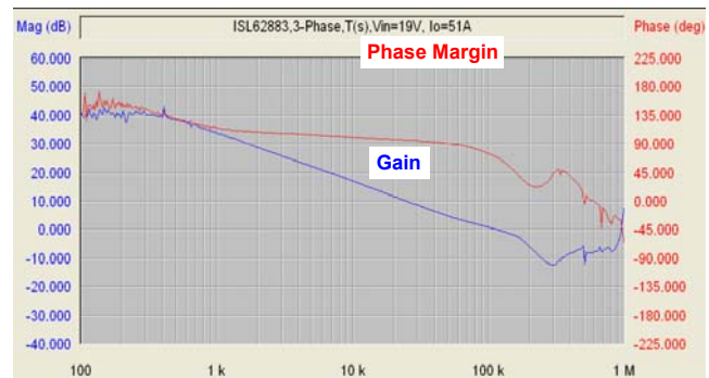
FIGURE 57. REFERENCE DESIGN LOOP GAIN T2(s) MEASUREMENT RESULT
