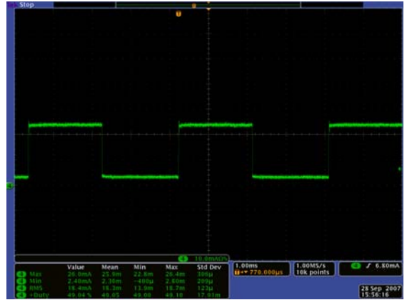
FIGURE 15. I LED AT 50% PWM DIMMING
