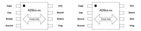
Pin configuration and sensitivity direction for the AD0xx-10 TDFN6 package are defined in the drawing below:
