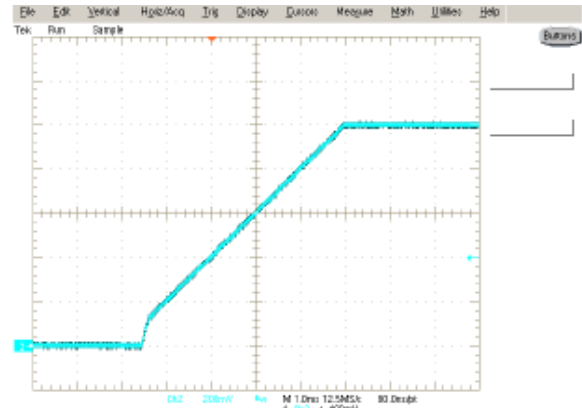
Figure 11: Turn on, V_{in}=8.0V , Load: 40A, CH2: V_{out}
