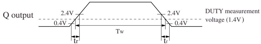
**Output duty cycle (CMOS)**
