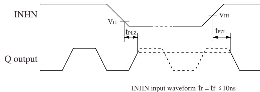
Note (AL $\times$  series only): when the device is in standby, the oscillator stops. When standby is released, the oscillator starts and stable oscillator output occurs after a short delay.
