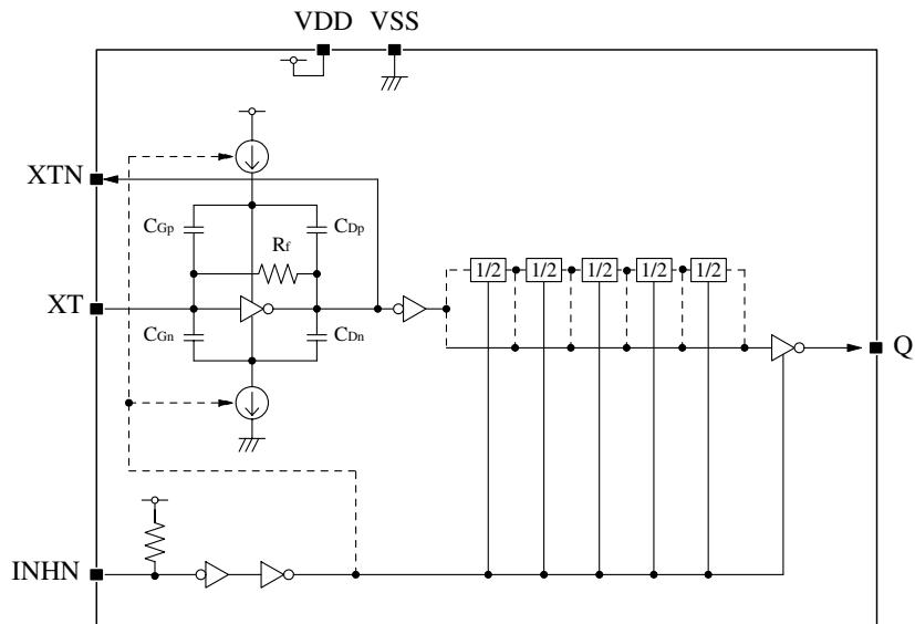
Notes. The SM5009 series reduce crystal current by limiting driving current of oscillating-stage inverter and inhibiting oscillating amplitude. Depending on the characteristics of using crystal or the mounting condition, they may not oscillate normally. Please evaluate the oscillation start-up characteristics adequately with your actual device.
