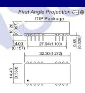
RECOMMENDED FOOTPRINT Top view,grid:2.54mm(0.1inch) diameter:1.00mm(0.039inch)
