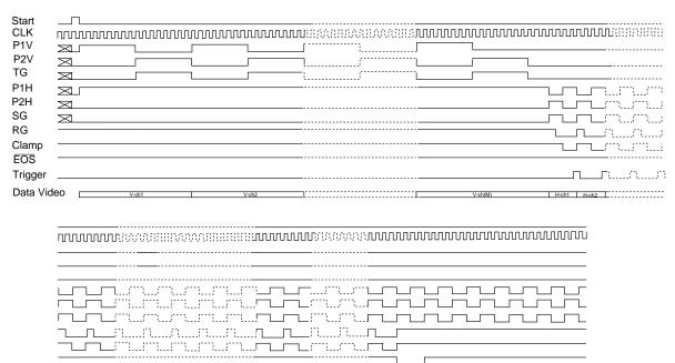
M=128, 256, 512 N=1044, 2068 V-ch1--V-ch2, V-ch (M-3)--V-ch (M): Isolation pixels H-ch1--H-ch4, H-ch (N-3)--H-ch (N): Blank pixels
