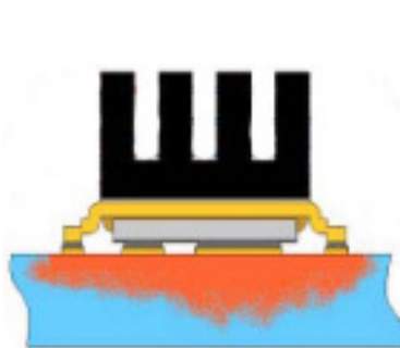
⑧ Mounted to a PCB with small clip heatsink (still air)
