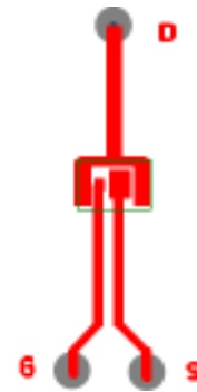
⑧ Mounted on minimum footprint full size board with metalized back and with small clip heatsink (still air)
