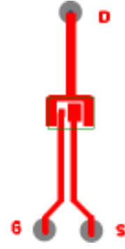
⑥ Mounted on minimum footprint full size board with metalized back and with small clip heatsink. (still air)
