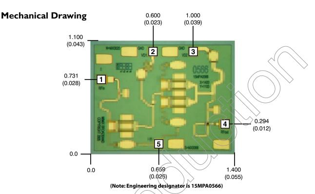
Units: millimeters (inches) Bond pad dimensions are shown to center of bond pad. Thickness: 0.110 +/- 0.010 (0.0043/4/z 0.0004), Backside is ground, Bond Pad/Backside Metallization: Gold All DC Bond Pads are 0.100 x 0.100 (0.004 x 0.004). All RF Bond Pads are 0.100 x 0.200 (0.004 x 0.008) Bond pad centers are approximately 0.109 (0.004) from the edge of the chip. Dicing tolerance: +/- 0.005 (+/- 0.0002). Approximate weight: 1.810 mg.
