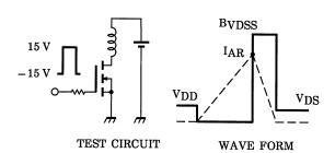
$$\begin{aligned} &R_G = 25~\Omega \\ &V_{DD} = 90~V,~L = 9.6~mH \end{aligned} \qquad E_{AS} = \frac{1}{2} \cdot L \cdot I^2 \cdot \left( \frac{BVDSS}{BVDSS - V_{DD}} \right) \end{aligned}$$
