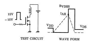
$$\begin{aligned} R_G &= 25 \ \Omega \\ V_{DD} &= 50 \ V, \ L = 1.48 \ mH \end{aligned} \qquad EAS = \frac{1}{2} \cdot L \cdot I^2 \cdot \left( \frac{BVDSS}{BVDSS - VDD} \right)$$
