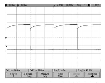
14. This effect is only apparent when driving high currents and only occurs on the rising edges. On the schematic in "Typical Application for a SPDT Switch" note that the rising edge turns on the shunt diodes. There will be a slight effect on isolation over time, but the insertion loss should not be affected.
