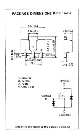
The 2SK680A, N-channel vertical type MOS FET, is a switching device which can be driven directly by the output of ICs having a 5 V power source.
