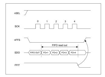
During FIFO access  $f_{SCK}$  cannot be higher than  $f_{ref}/4$ , where  $f_{ref}$  is the crystal oscillator frequency.
