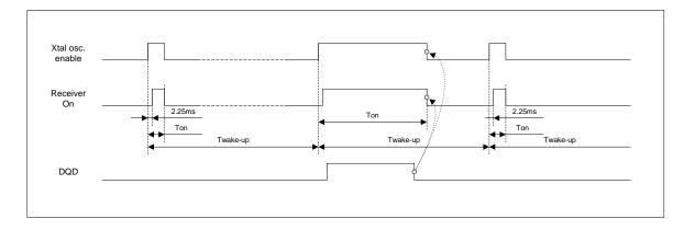
Bit O (en): Enables the Low Duty-Cycle Mode. Wake-up timer interrupt not generated in this mode.
