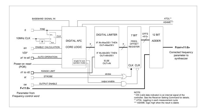
Note: Lock bit is high when the AFC loop is locked, f\_same bit indicates when two subsequent measuring results are the same, toggle bit changes state in every measurement cycle.
