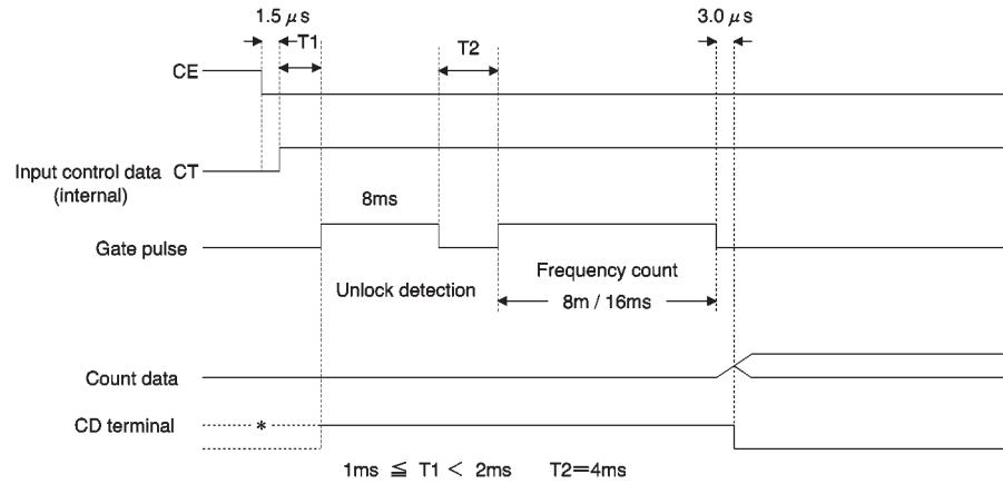
(2) When CT = 0 and GT = 1: Only unlock detection is carried out.
