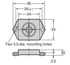
Case material: ABS resin Filling: Epoxy resin
