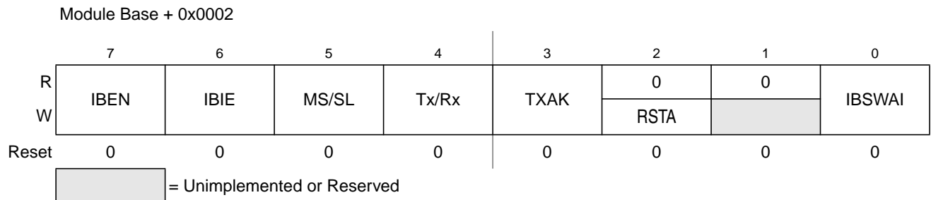
Figure 10-6. IIC Bus Control Register (IBCR)
