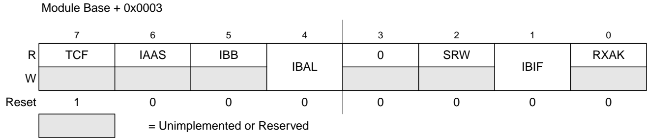
Figure 10-7. IIC Bus Status Register (IBSR)
