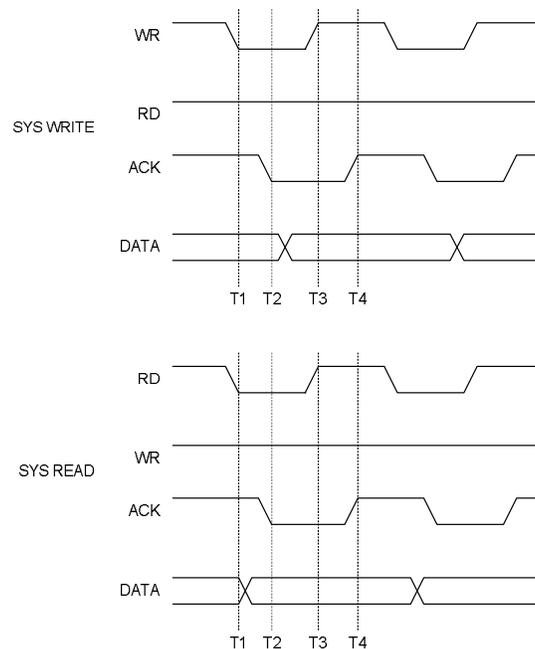
WR, RD are output from system CPU and ACK is output from SC9645 ,the default signal level is high and DATA bus can be used by system CPU and SC9645.
