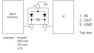
\* We recommend using pin-1 as input port.
