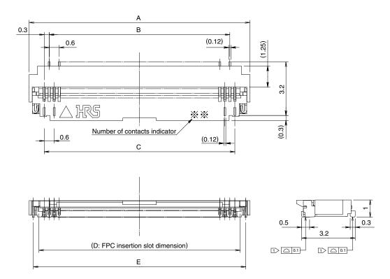
Notes 1 The coplanarity of each terminal lead within specified dimension is 0.1 mm Max.
