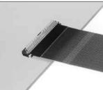
Rotate down the actuator until firmly closed. It is critical that the inserted FPC is not moved and remains fully inserted.
