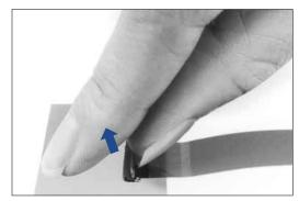
Fully insert the FPC in the connector parallel to mounting surface, with the exposed conductive traces facing down.
