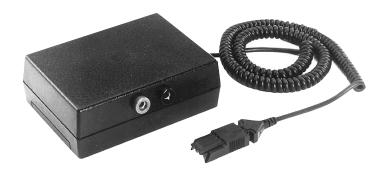
The MOD400R Field Sensitivity Test Module can be used with any standard DC voltmeter or multimeter to check the sensitivity range of System Sensor detectors (satisfies NFPA 72 requirement for sensitivity testing).
