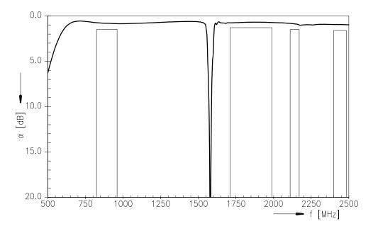
GPS - NON-GPS (isolation, transfer function for matching circuit 1, all bands):
