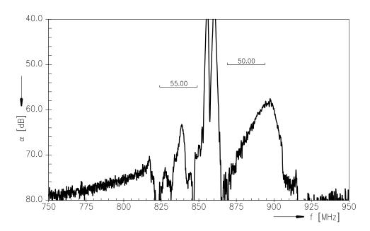
Frequency Response TX-RX (Wideband Differential Mode Isolation)
