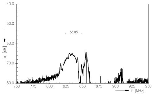
Frequency Response TX-RX (Wideband Common Mode Isolation)
