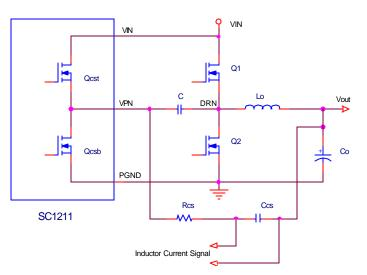
The above circuit shows the concept of Combi-Sense™ technique. An internal totem pole (Qcst, Qcsb) generates a VPN (Virtual Phase Node) signal. This VPN follows
