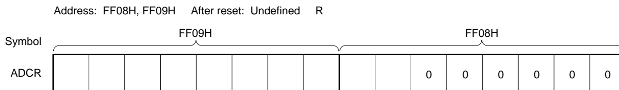
Figure 12-6. Format of A/D Conversion Result Register (ADCR)
