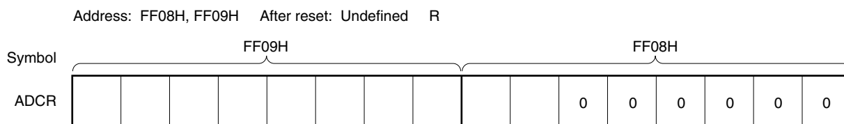
Figure 12-6. Format of A/D Conversion Result Register (ADCR)
