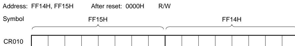
Figure 6-4. Format of 16-Bit Timer Capture/Compare Register 010 (CR010)
