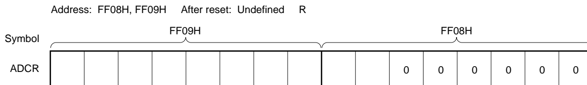
Figure 10-6. Format of A/D Conversion Result Register (ADCR)
