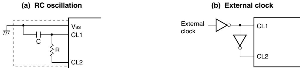
Figure 5-10. External Circuit of External RC Oscillator
