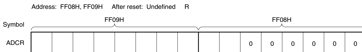
Figure 11-6. Format of A/D Conversion Result Register (ADCR)
