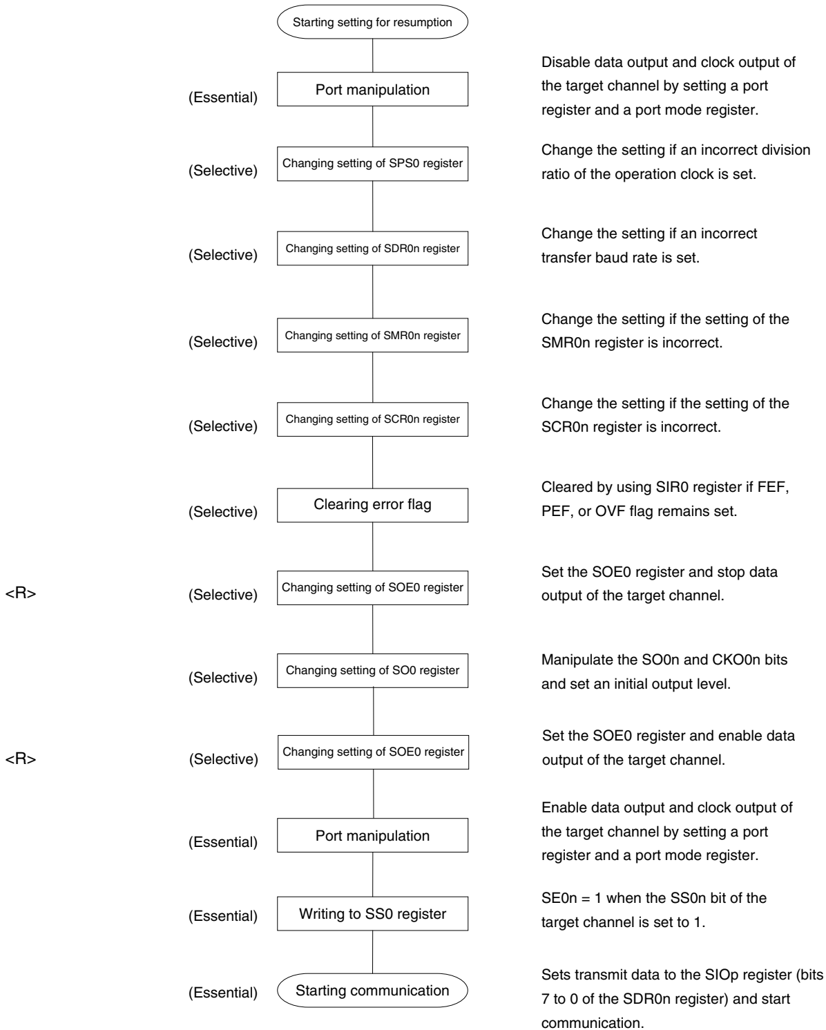
Figure 11-41. Procedure for Resuming Master Transmission/Reception
