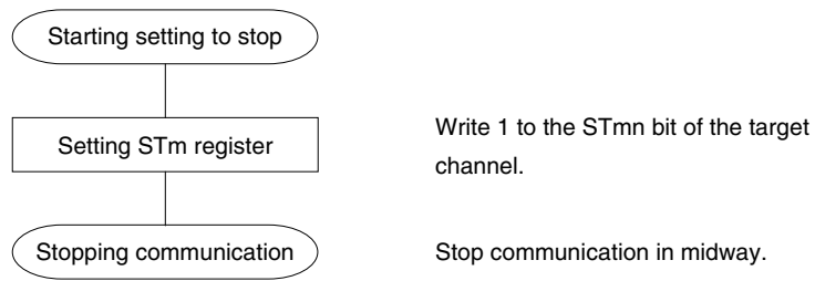
Figure 11-70. Procedure for Stopping UART Transmission
