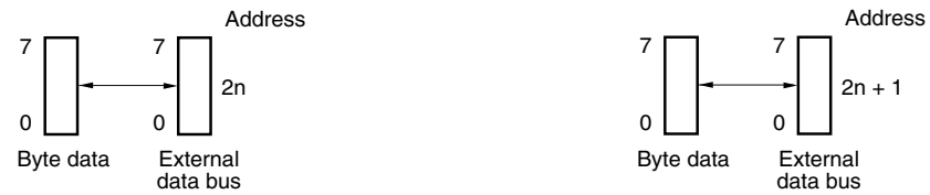
Figure 7-21 Left: Access to even address ( 2n ) Right: Access to odd address ( 2n + 1 )
