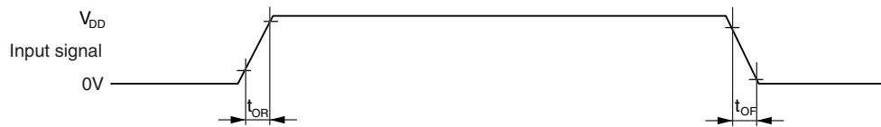
Figure 27-5: Output Rise and Fall Time
