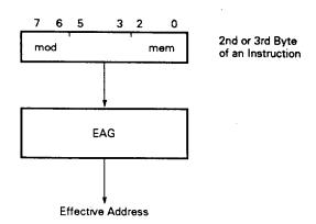
If it reads the byte (the 2nd or 3rd byte) specified by the instruction's operand and requires memory access, it will generate a control signal related to the ALU and the associated register operation, and will calculate an effective address to transfer the signal to the DP (Data Pointer).
