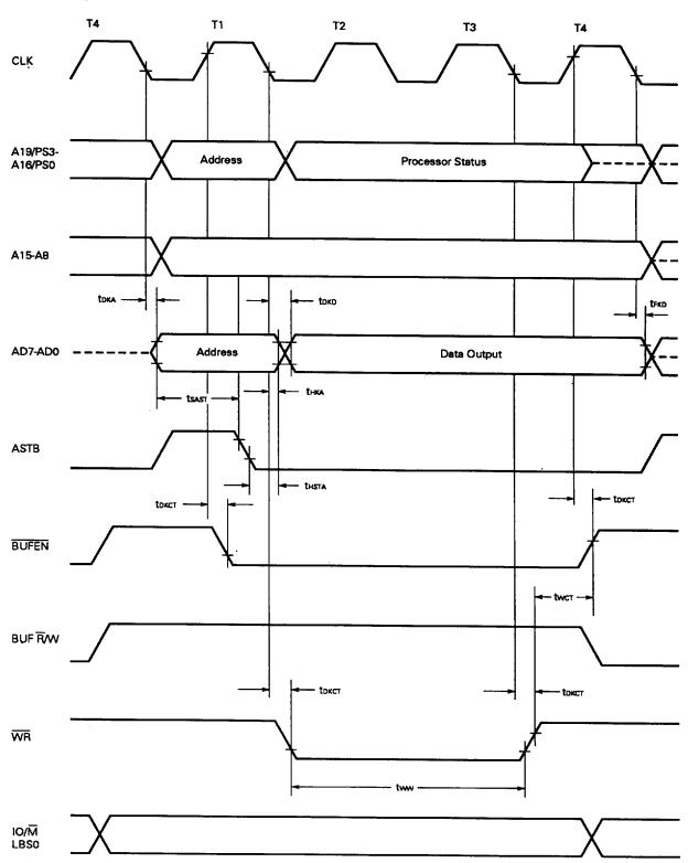
Remark A broken line shows high impedance.
