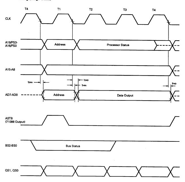
Remark A broken line shows high impedance.
