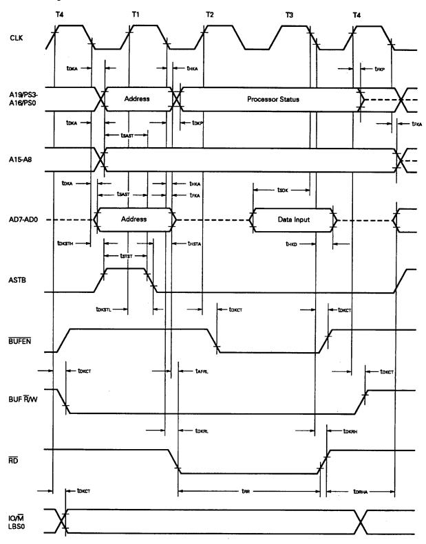
Remark A broken line shows high impedance.
