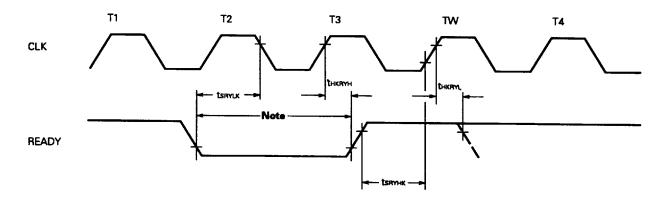
Note It is necessary to fix the READY signal to low (or to high) during this period.
