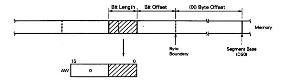
Bit field data can extend over the byte boundaries of memory.
