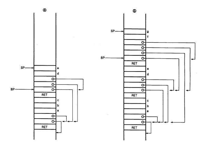
The PREPARE instruction saves BP to a stack first in order to restore the BP of a procedure at the called side when the procedure finishes. Then, it pushes a frame pointer (a saved BP) onto the stack within the range accessible from the called procedure. The accessible range equals to the value which is subtracted by one from the lexical level of the procedure.
