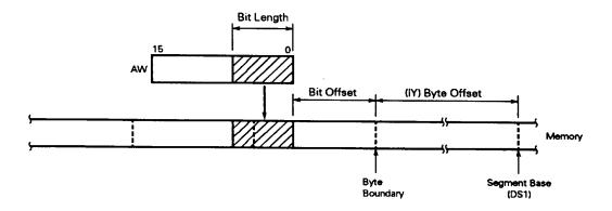
Bit field data can extend over the byte boundaries of memory.
