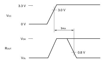
Receiver outputs are indefinite during reset release time (tpra).
