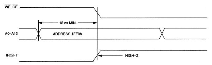
The  $\overline{IRQ}/FT$  pin can also be activated in the battery-backed mode. The  $\overline{IRQ}/FT$  will go low if an alarm occurs and both ABE and AE are set. The ABE and AE bits are cleared during the power-up transition, however an alarm generated during power-up will set AF. Therefore the AF bit can be read after system power-up to determine if an alarm was generated during the power-up sequence. Figure 4 illustrates alarm timing during the battery backup mode and power-up states.
