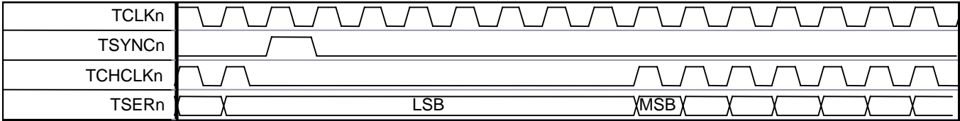
Figure 11-31. E1 Transmit-Side TCHCLKn Gapped Mode During Channel 1
