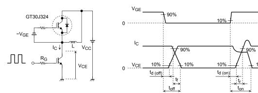
Note 2: Switching loss measurement waveforms
