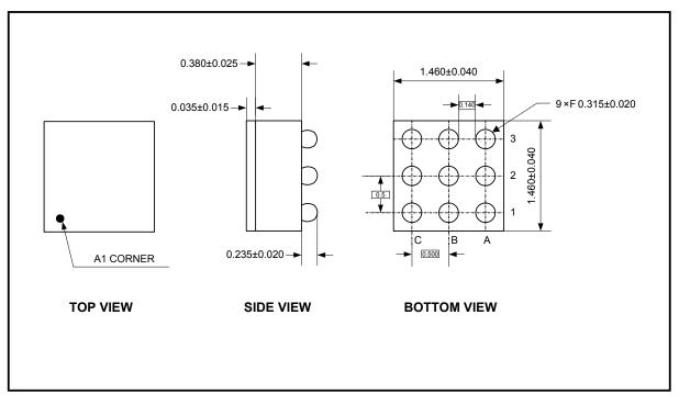
Note: All linear dimensions are in millimeters.
