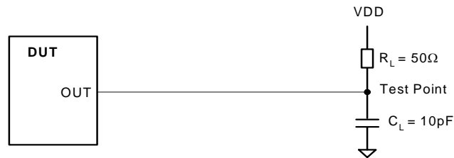
Figure 19. Load Circuit - High to Low Slew Measurement
