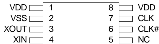
Figure 1. Pin Diagram - 8-Pin TSSOP
