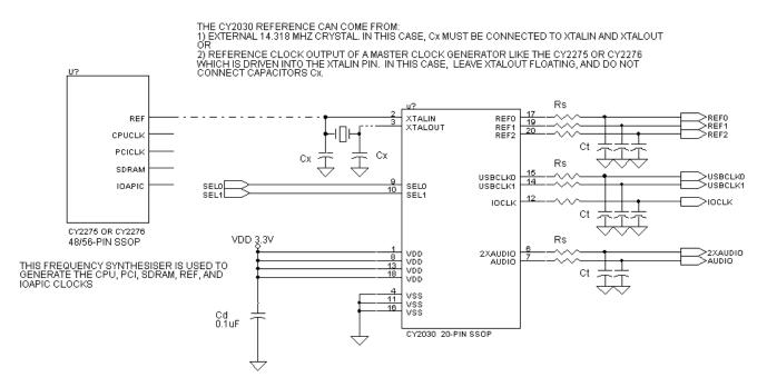
CX = LOAD MATCHING CAPACITORS, REQUIRED WITH EXTERNAL CRYSTALS = 2 \* CRYSTAL LOAD CAPACITANCE
