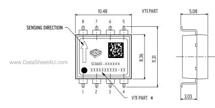
Acceleration in the direction of the arrow will increase the output voltage.
