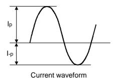
Unbalance rate =  $| I_p - I_{-p} | / I_L \times 100$  (%) Wave-height rate =  $I_p$  (or  $I_{-p}$ ) /  $I_L$
