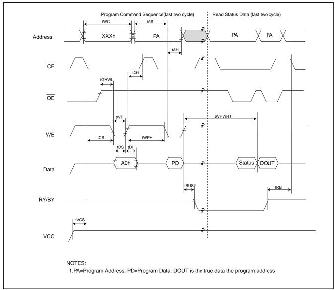
Fig 10. Accelerated Program Timing Diagram
