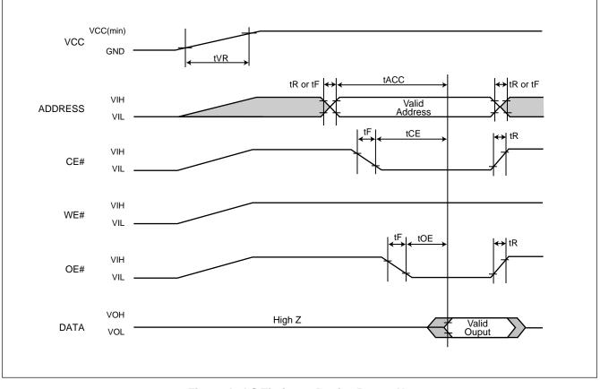
Figure A. AC Timing at Device Power-Up
