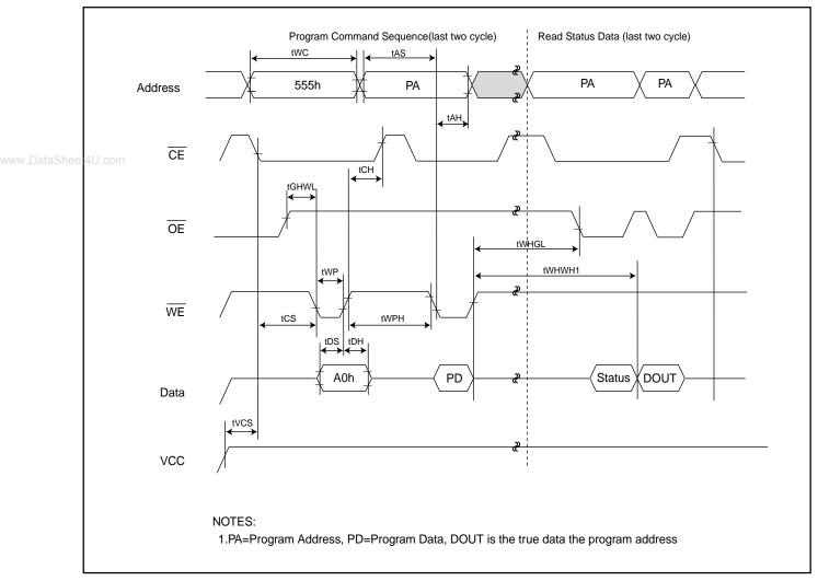
Fig 7. Accelerated Program Timing Diagram
